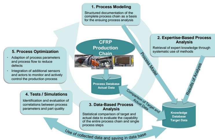
**Figure 1:** Methodical approach to model, analyze and optimize CFRP production processes
