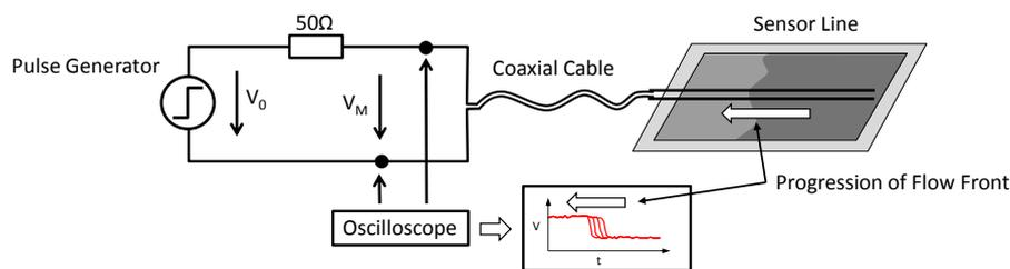
Figure 2: TDR sensor setup
